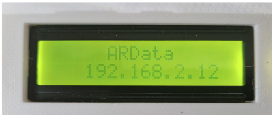
Note: If after 30 seconds the device has not displayed an IP Address, check connectivity to the ethernet port **or** change the power source connection as the AR Data relay unit may not have sufficient power.
